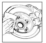
9. Remove any rust or dirt from the wheel bolts, mounting surfaces and spare wheel.
